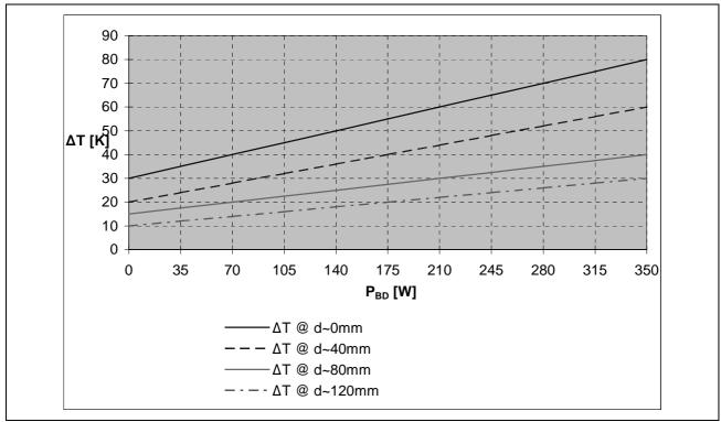
P<sub>BD</sub>: average continuous power of braking resistor
