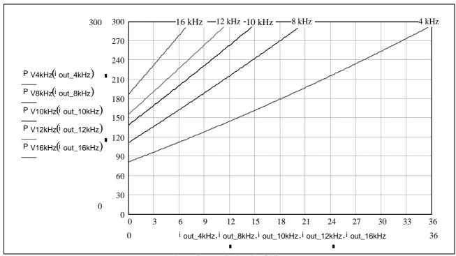
Fig. 6-19: Power dissipation power section HCS02.1E-W0070
