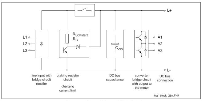
Fig. 1-5: HCS02.1E-W0028-NNNN - Block diagram
