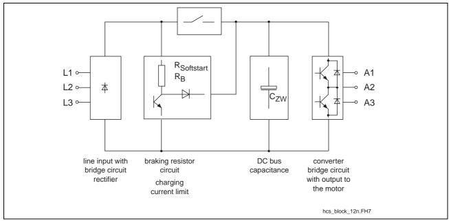
Fig. 1-3: HCS02.1E-W0012-NNNN - Block diagram
