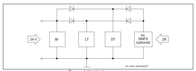
Br: brake circuit LT: power section ST: control section
