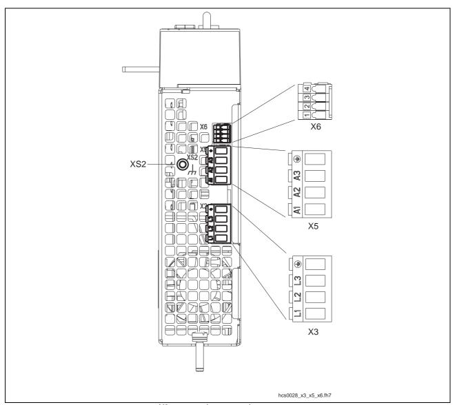
X3: mains connection X5: motor connection
