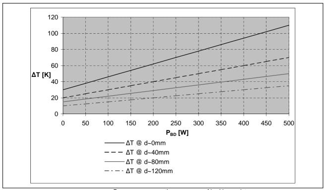
P<sub>BD</sub>: average continuous power of braking resistor
