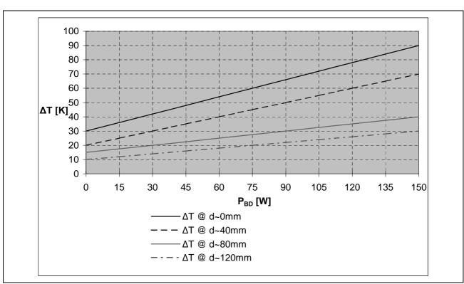
P<sub>BD</sub>: average continuous power of braking resistor
