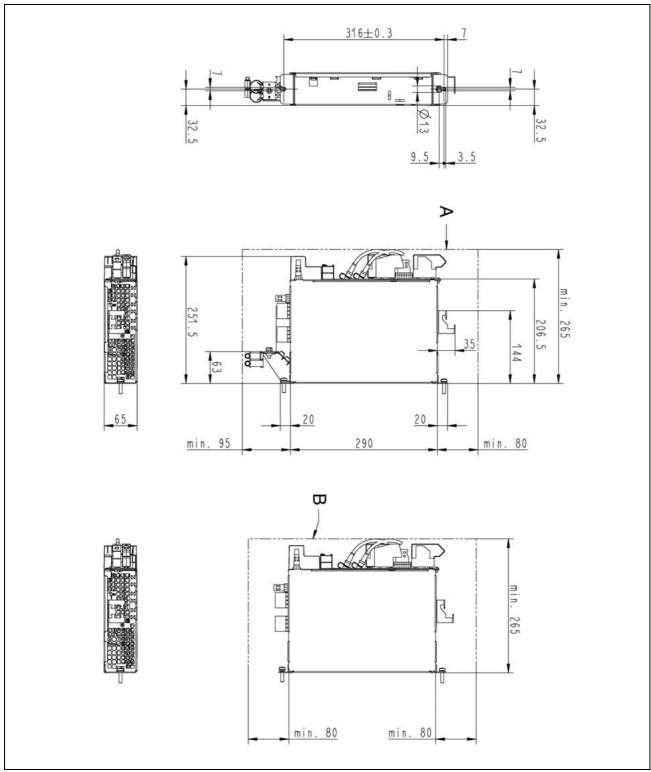
A: minimum mounting clearance (when using accessories HAS02.1); plus space for cables
