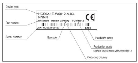
Fig. 4-3: Type plate power section
