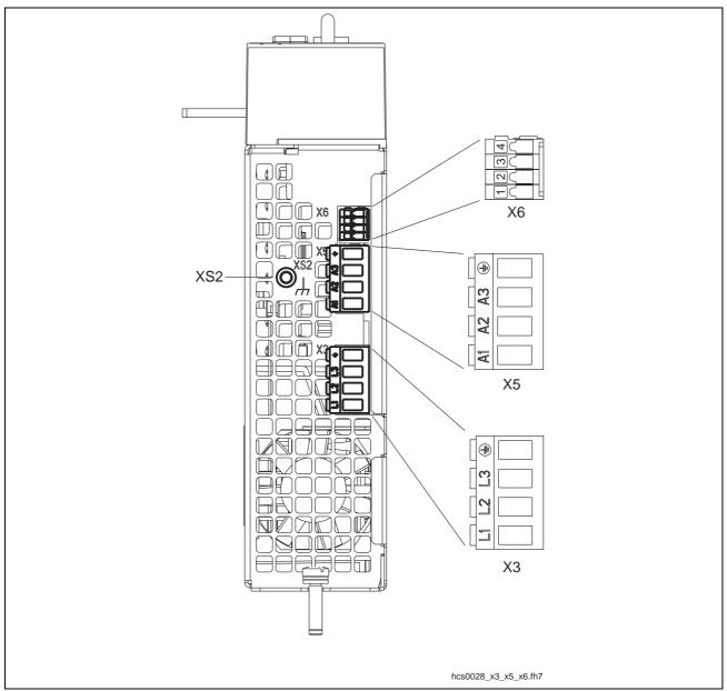
X3: mains connection X5: motor connection
