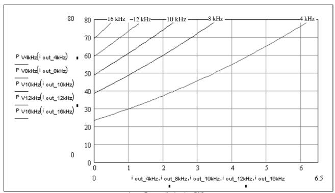
Fig. 6-16: Power dissipation power section HCS02.1E-W0012
