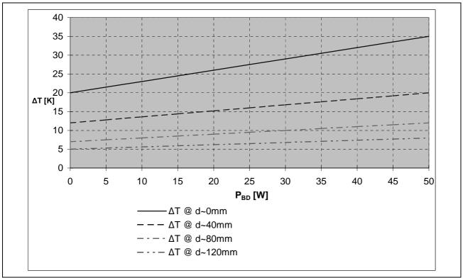
P<sub>BD</sub>: average continuous power of braking resistor
