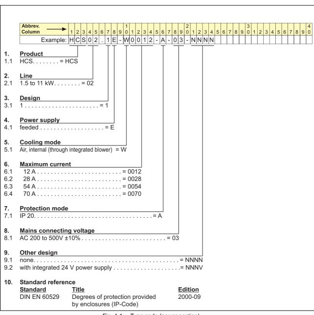
Fig. 4-1: Type code (power section)
