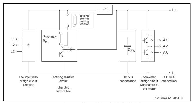
Fig. 1-7: HCS02.1E-W0054/70-NNNN - Block diagram
