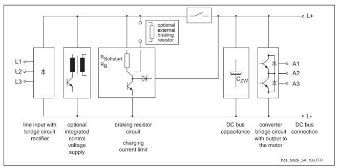
Fig. 1-8: HCS02.1E-W0054/70-NNNV - Block diagram
