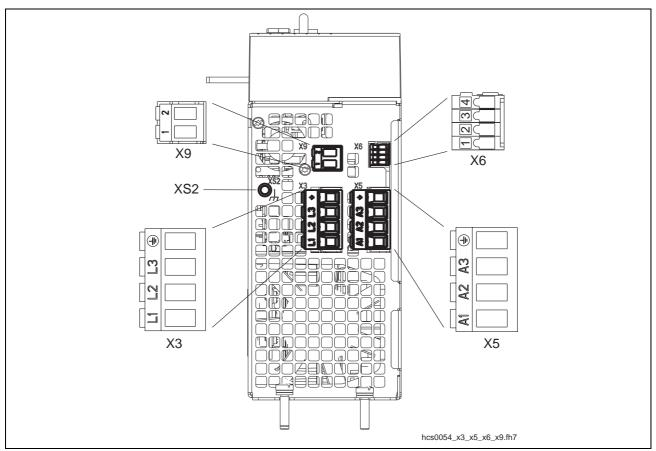
X3: mains connection X5: motor connection
