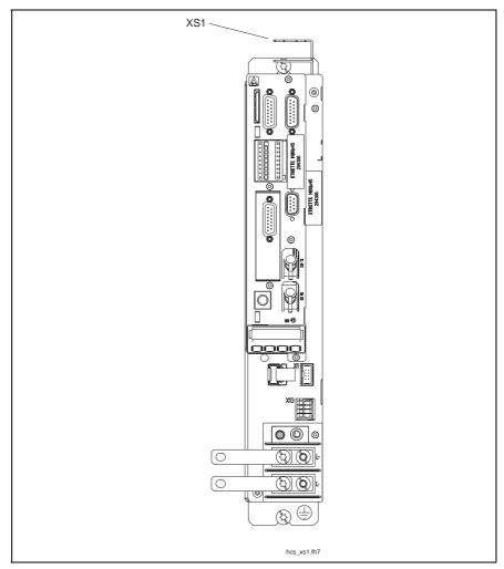
Fig. 6-54: Shield connection XS1
