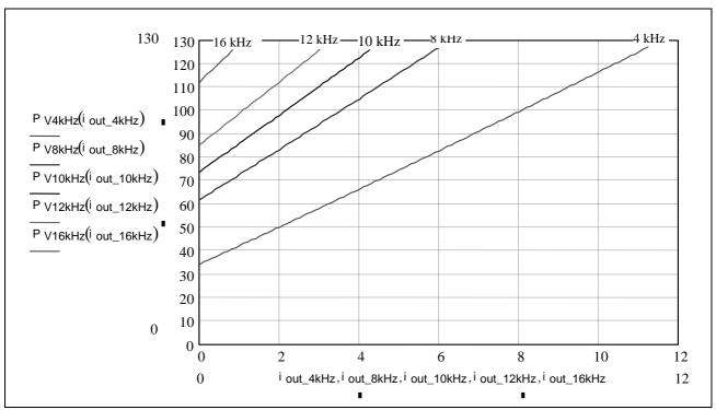
Fig. 6-17: Power dissipation power section HCS02.1E-W0028
