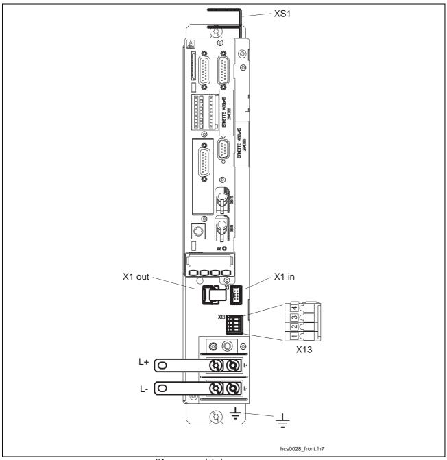
X1: module bus X13: control voltage
