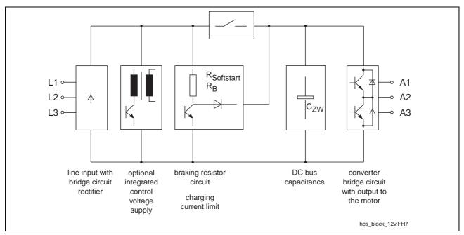
Fig. 1-4: HCS02.1E-W0012-NNNV - Block diagram
