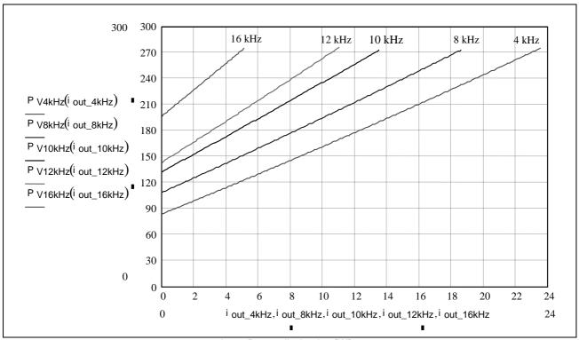
Fig. 6-18: Power dissipation power section HCS02.1E-W0054
